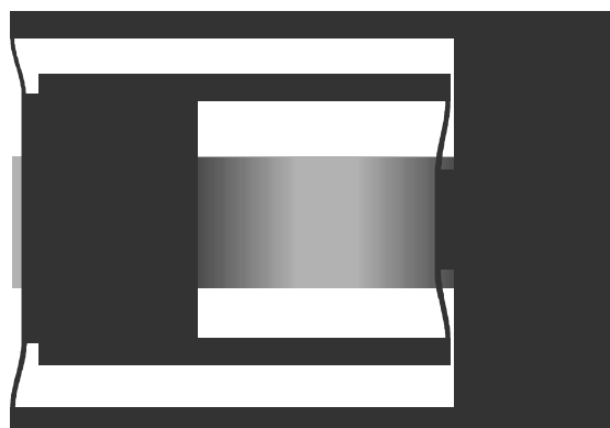
Figure 6.5: Deformation of the connection springs due to contraction of the plate (the step size has been exaggerated). Both the bending stiffness and the connection springs push the two frame parts apart when the plate is released.
