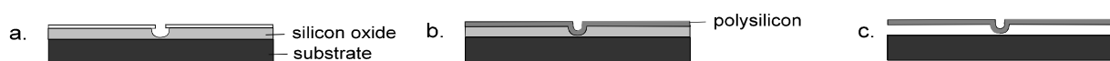
Figure 3.11: Fabrication of bumps according to [48, 49]. a) isotropic etch of hole b) deposit polysilicon structural layer c) release etch.
